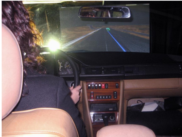
Figure 11. View of driving simulator from inside test vehicle.
