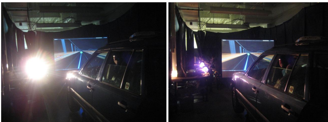
Figure 7. Comparison of light transmittance through in-phase (left) and out-of-phase (right) polarizing filter over camera lens.
