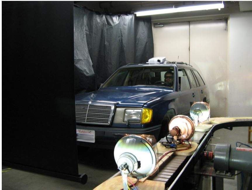
Figure 5. Headlights on moving conveyor belt simulating oncoming traffic.
