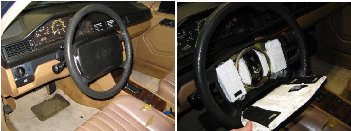
Figure 8. Installation of gyroscopic mouse into faux-airbag.
