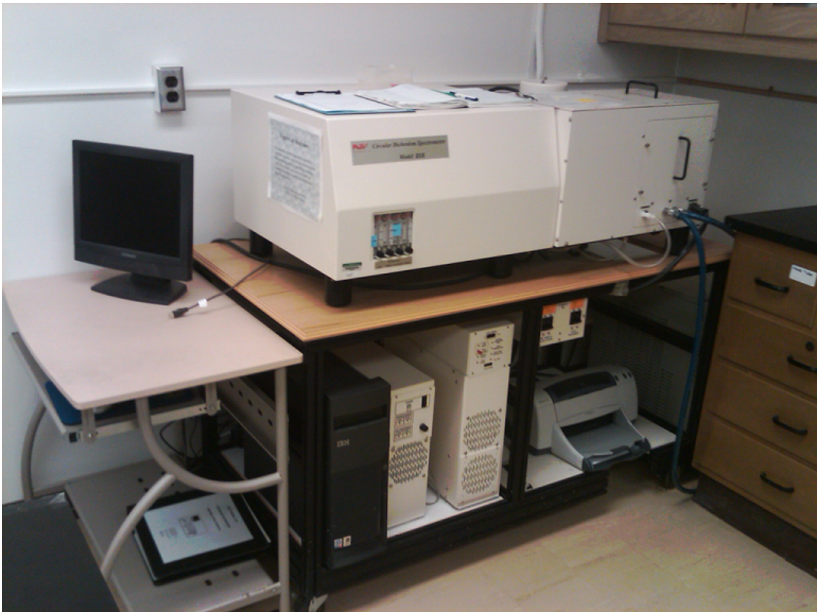
Figure 1-9. Aviv model 215 circular dichroism instrument (New Jersey, USA) used in this study.
