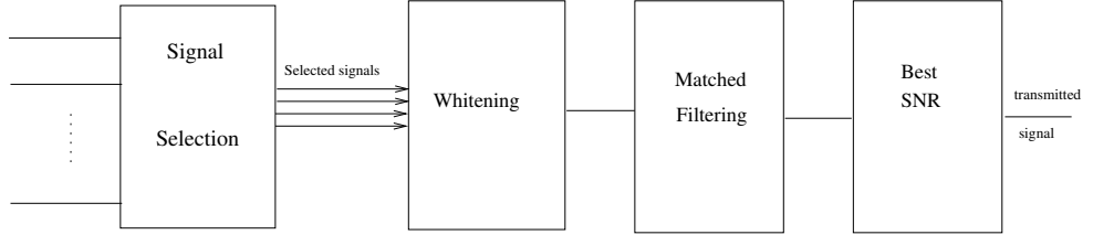
Figure 3.10. Optimum relay processing during m 'th time slot
