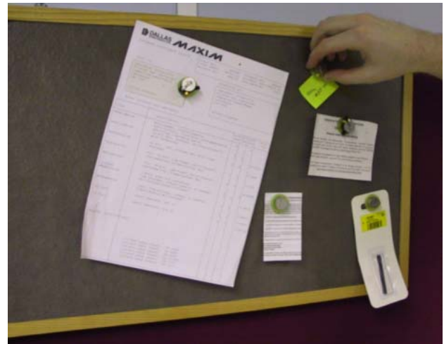
Figure 4. The Pin&Play pins are used as normal pins, the Pin&Play surface provides them with power and networking. The pins' batteries allow them to be moved from one board to another without losing any information.
