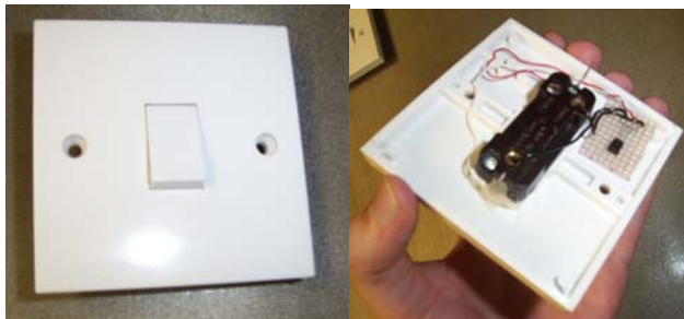
Figure 6. The front (left) and internals (right) of a Pin&Play wall switch.
