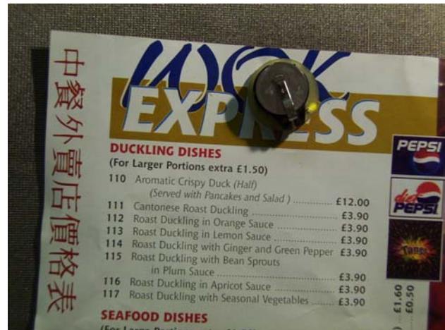
Figure 5. The pin's internal clock and calendar allow the pin to notify the user(s) when its document becomes invalid by lighting up its LED.
