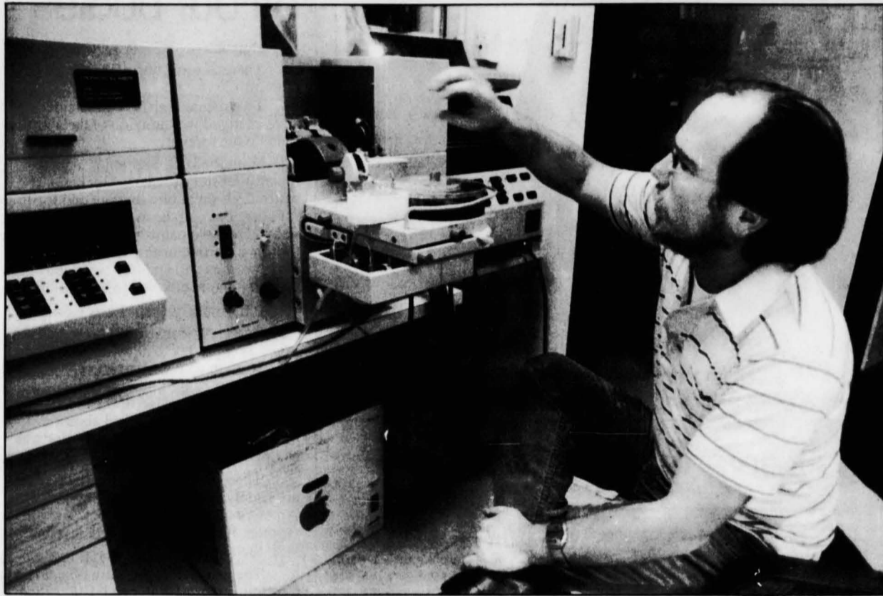
Michael Gordon, an SJSU graduate, dries up organic material for study in the atomic absorption spectrophotometer
