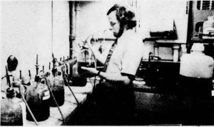
SJSU Civil Engineering professor Robert Fisher is producing methane gas in 4-liter jugs containing scraps of onions and garlic, water and sewage bacteria.
