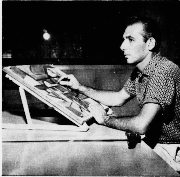
INVENTOR Humbert G. Miraglia Jr. demonstrates a Tilt A Table, a device he invented in an SJS industrial design class last semester. The drawing board adapter enables the user to have his work at the desired angle.
