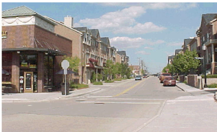
Figure 4-10: Innovative Character of Housing--the 3-story housing units are stacked with a one-level unit on the 1st floor, and a two-level unit starting on the 2nd floor. One can also see a local store on the left side of the image.
