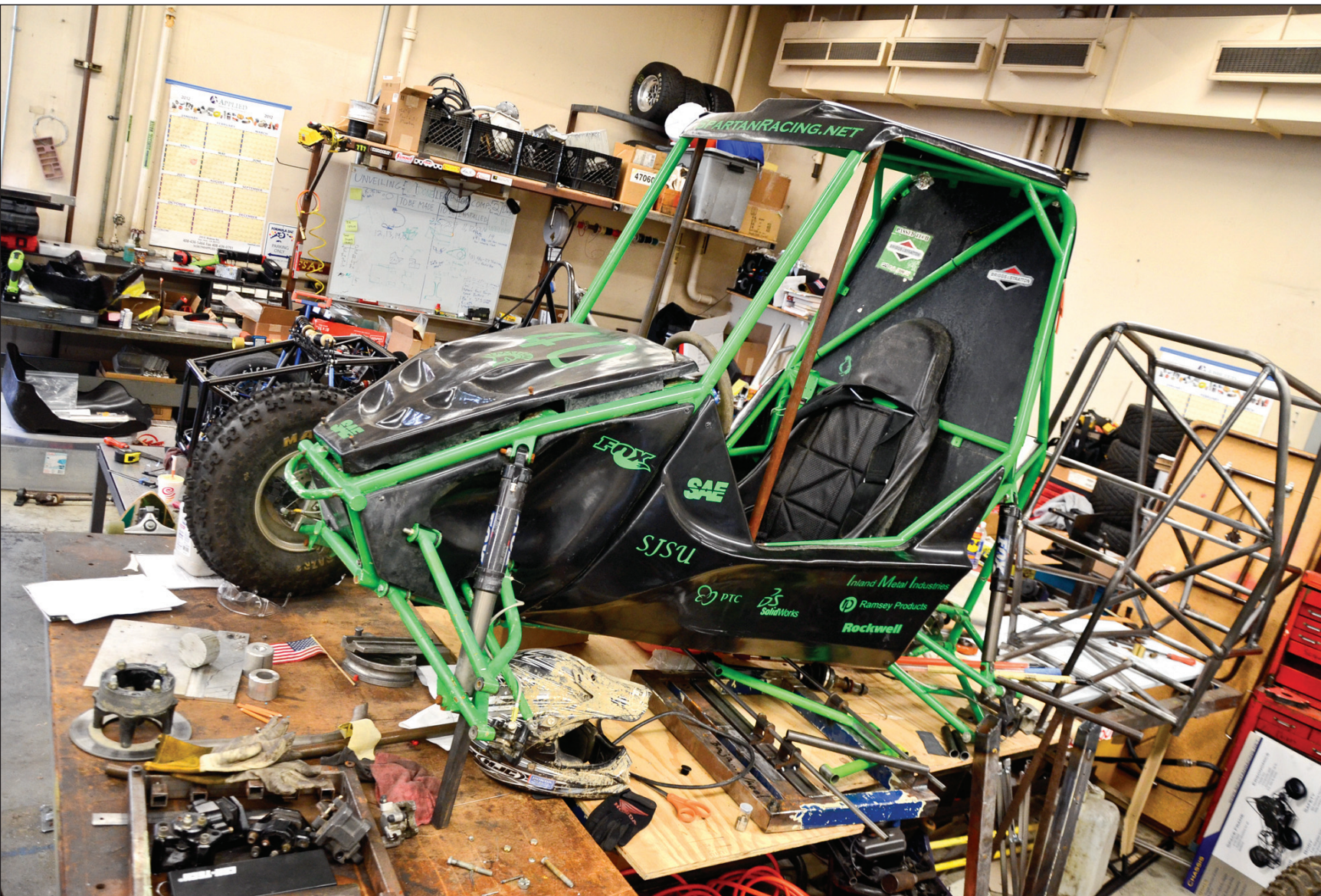
The SJSU Spartan Racing SAE Baja chassis is being upgraded with reinforced suspension components in the Engineering building garage. Designed to bump over rocks and smash through the mud, the unofficial motto of the Baja Team is design, build, destroy, rebuild. Photo by Jasper Rubenstein / Spartan Daily
