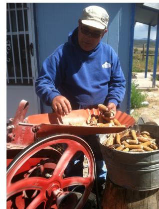
Figure 7. Desgranando los chicos . The author uses a home-made machine to strip the kernels from the roasted chicos cobs. A few remnant kernels must be stripped by hand. This machine was adapted by another local farmer and he calls it adesgranador . Cornelio Arellano Home, Cuba neighborhood, San Luis, CO, Sept. 2014. Photo by E. H. Peña.
