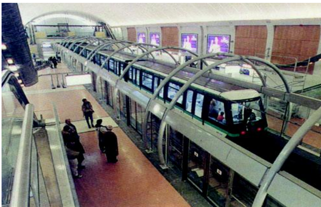
Figure 9. Passenger Separation System on Paris Meteor
