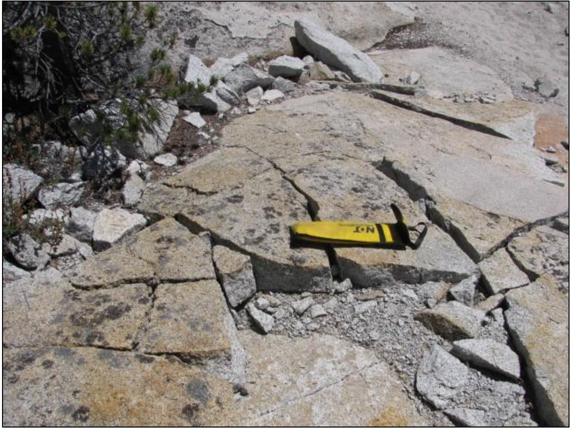
Figure 20. Photo illustrating in situ blocks with joint spacing < 1 m with glacial polish on their surfaces indicating they were either not moved during glaciation or joints formed post-glacial.
