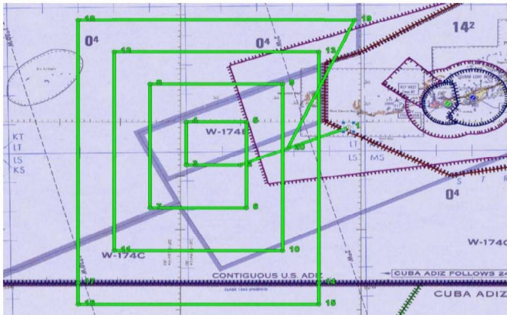
Figure 9. UAS Flight Path Example. This image shows the planned route of a ScanEagle UAS in a green corkscrew pattern performing a marine fisheries protection and monitoring operation. Image reproduced with permission from RTCA, Inc. Copyright 2010 by RTCA, Inc. 1
