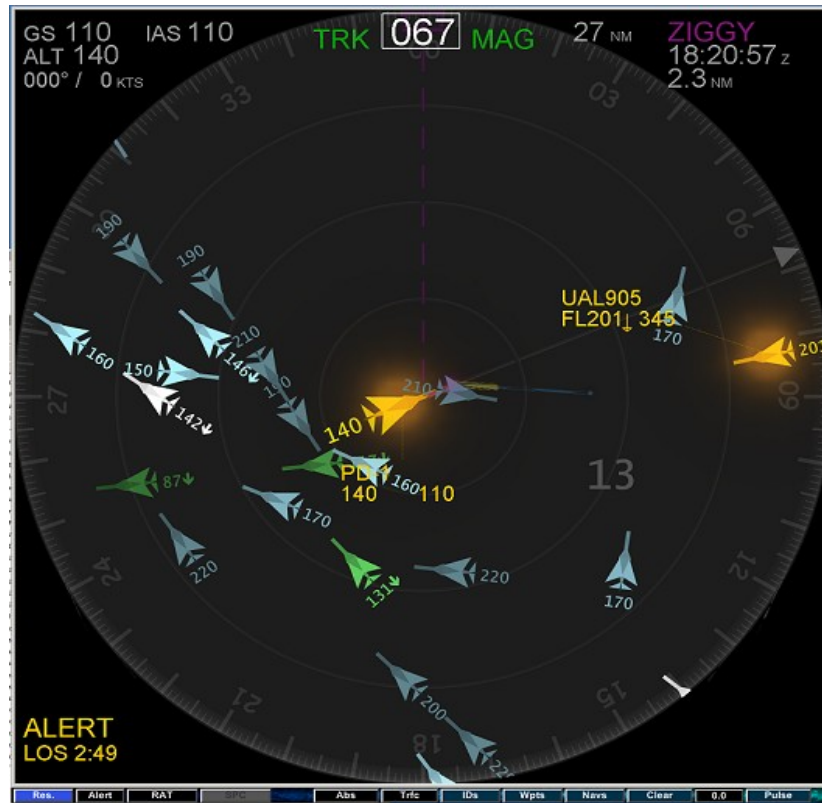
Figure 11. The Ames 3D CSD. Green aircraft were 500+ ft below ownship's altitude, white aircraft were within 500 ft above or below ownship's altitude, and blue aircraft were 500+ ft above ownship's altitude. The visual alert of the yellow glowing ownship and intruding aircraft can be seen indicating a conflict.
