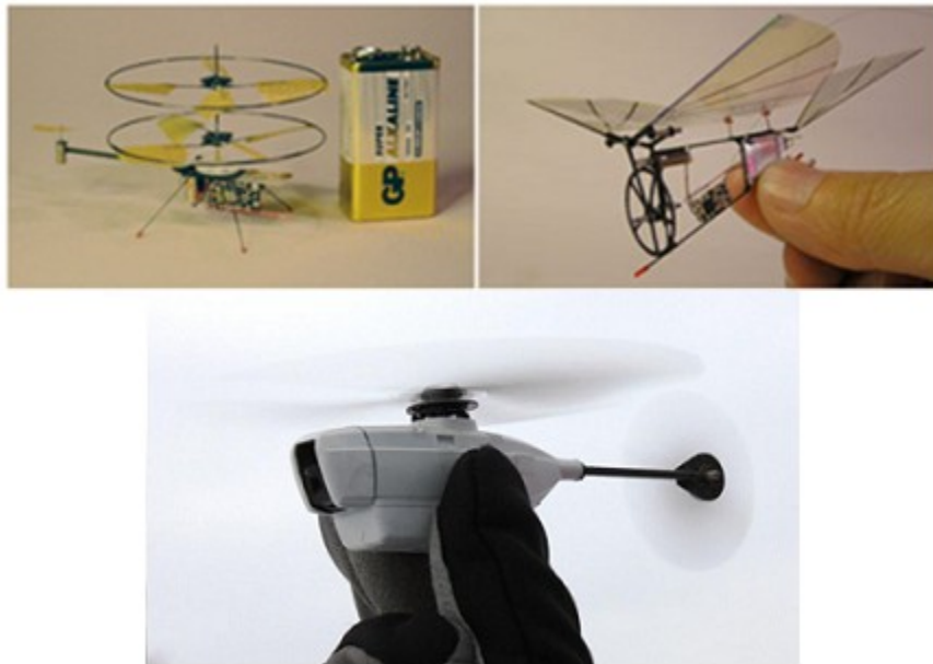
Figure 5. Nano Air Vehicles. Examples of NAVs include the Pico-flyer (top left), the Ornithopter (top right), and the PD-100 Black Hornet (bottom). Image reproduced with permission from Prox Dynamics. Respective copyrights 2005, 2007, and 2009 by Prox Dynamics.
