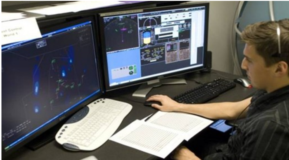
Figure 12. MACS in Pseudo Pilot Mode. MACS allowed the pseudo pilots to control multiple aircraft at a time through the use of automation. The monitor on the left displays the sector, and the monitor to the right displays aircraft controls.
