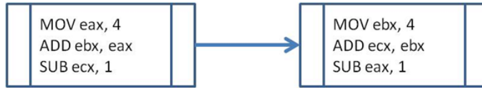
Figure 3: Register renaming example.
