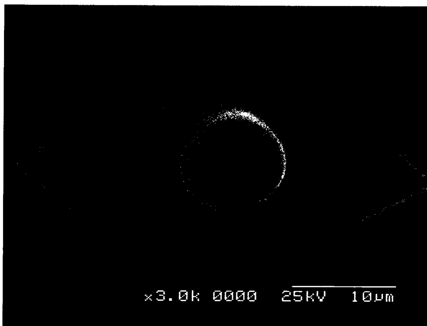
Figure 33. SEM image of probe after dip-coating in 3,200 ppm Cloisite® 25A – NMP. The borosilicate particle appears fuzzier after dip-coating in the 3,200 ppm solution. The fuzziness may be an indication of a coating of Cloisite® 25A.
