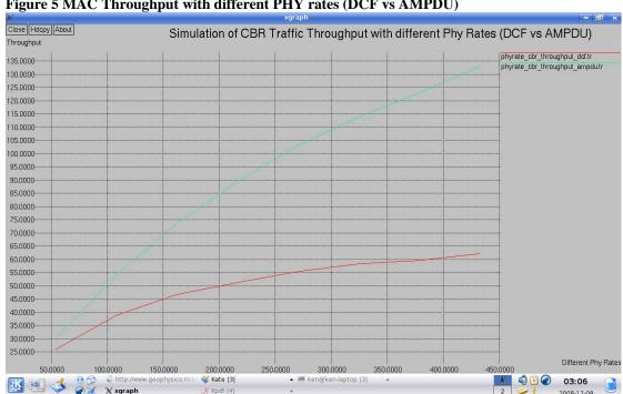
Figure 5 MAC Throughput with different PHY rates (DCF vs AMPDU)
