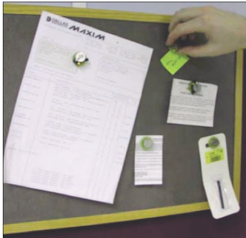
■ Figure 4. The necessary data is stored locally in the pins, so they can be moved to a different board. The onboard battery enables the pins to retain their document's data (e.g., when it expires or how important it is).
