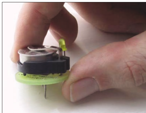
■ Figure 2. A close-up of an assembled pin. The current model has two isolated pins for accessing the top and bottom layers. The one-wire switch is hidden below the i-Button's connector, next to the LED.
