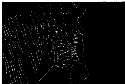
Figure 5.8: Intersection of Canny Edges in the Zebra Preprocessed with the Gaussian Filter
