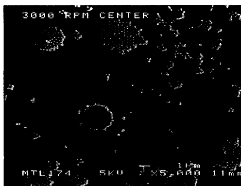
Figure 61. SEM image showing the silica nanosphere at the center of the sample prepared at 3k rpm.
