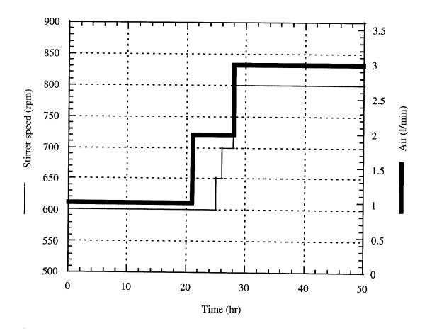
Figure 12. Operating conditions of stirrer speed and air flow rate vs. time for batch/fed-batch operation.
