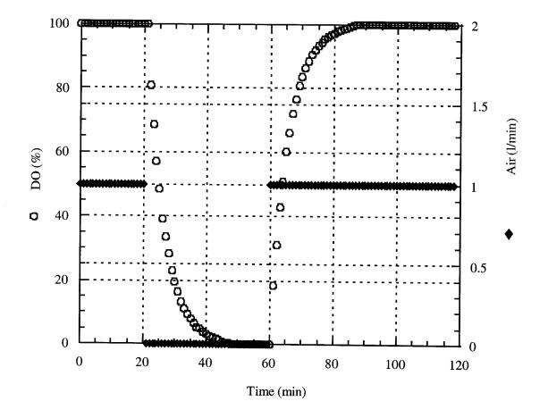
Figure 9. Oxygen transfer in a 3-liter bioreactor with one liter growth medium. The stirrer rate was fixed at 600 rpm.
