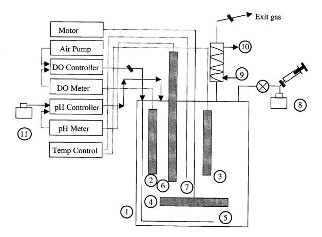
Figure 1. Typical bioreactor configuration (provided by Dr. Claire Komives)
