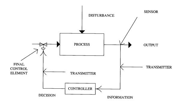
Figure 2. Feedback control loop.
