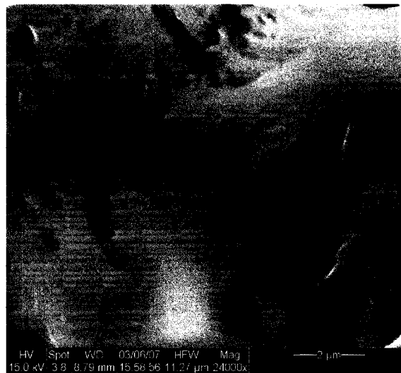
Figure 34. An SEM image of the template infiltrated with gel, partially dissolved then annealed to 600 °C and then again at 1000 °C.
