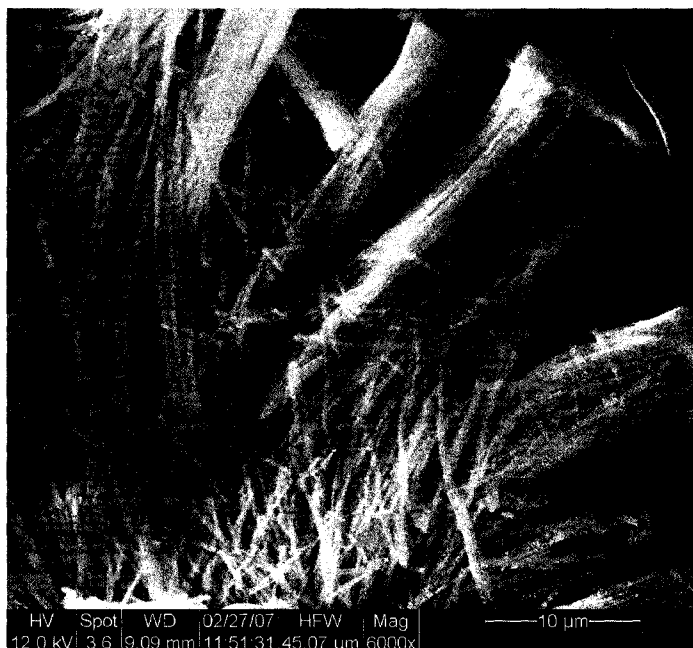
Figure 31. An SEM image of the dried nanowire gel attached to a partially dissolved alumina template.
