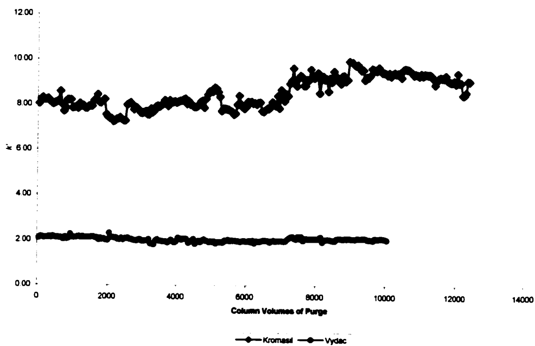
Figure 31. Plots of Pyrene Retention Factor versus Number of Mobile-Phase Volumes at pH 9-10. (After purging 7000-column volumes mobile phase, pH changed to 10). Mobile phase: 70:30 (v:v) methanol-water; flow rate: 0.7 mL/min; column temperature: room temperature (20~25 °C); detection: UV absorbance at 254 nm; sample volume 20 \mu L.
