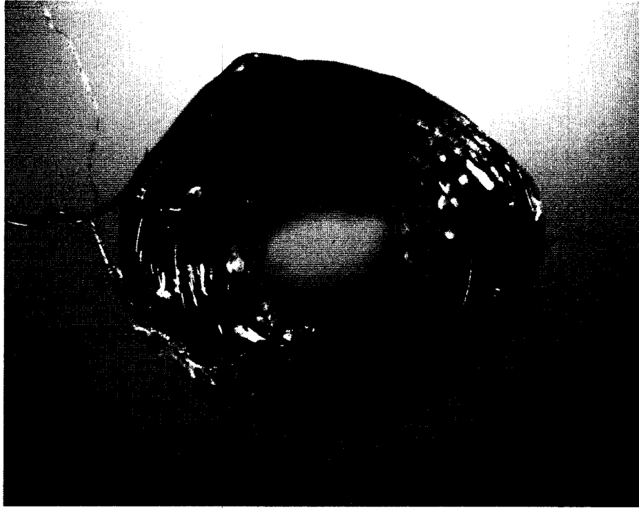
Figure 2. Scleral Search Coil . Coil was glued to the cornea over the pupil of the right eye. Copper wire coil (0.008 inch diameter, 100 turns, 1.0 mg approx.) held together with superglue
