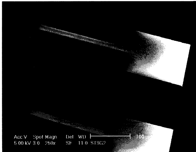
Figure 33. SEM image of 220 \mu\text{m} and 240 \mu\text{m} beam from wafer with polysilicon deposited at 620 ^{\circ}\text{C} with no annealing.
