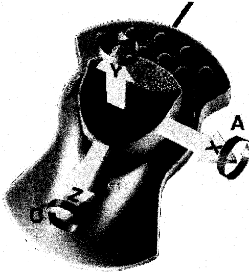
Figure 15. 3D Space Mouse. The 3D Space Mouse provided freedom of movement along the Y, X, and Z axis. However, the Z-axis was disabled because the task required only 2D movement.
