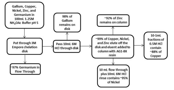
Figure 2 | Flow chart indicating the separation strategy to recover <sup>67</sup>Cu from the aqueous samples containing <sup>67</sup>Cu projectile fragments collected at the NSCL.
