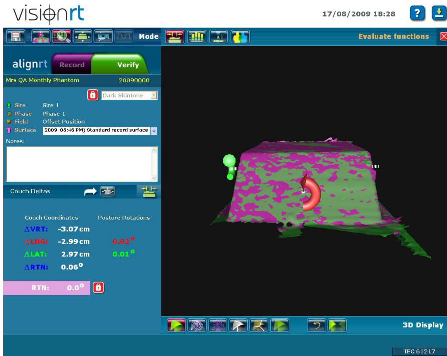
Fig. 3. Couch shifts determined by the AlignRT system (cm): -3.07 vertical, -2.99 longitudinally, and 2.97 laterally.
