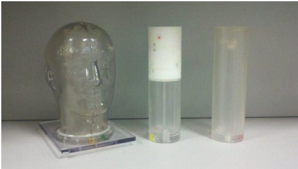
FIG. 1. The anthropomorphic outer shell to the phantom (left), the dosimetry insert containing radiochromic film and TLD (middle), and the modified imaging insert containing the target and OAR (right) are shown.
