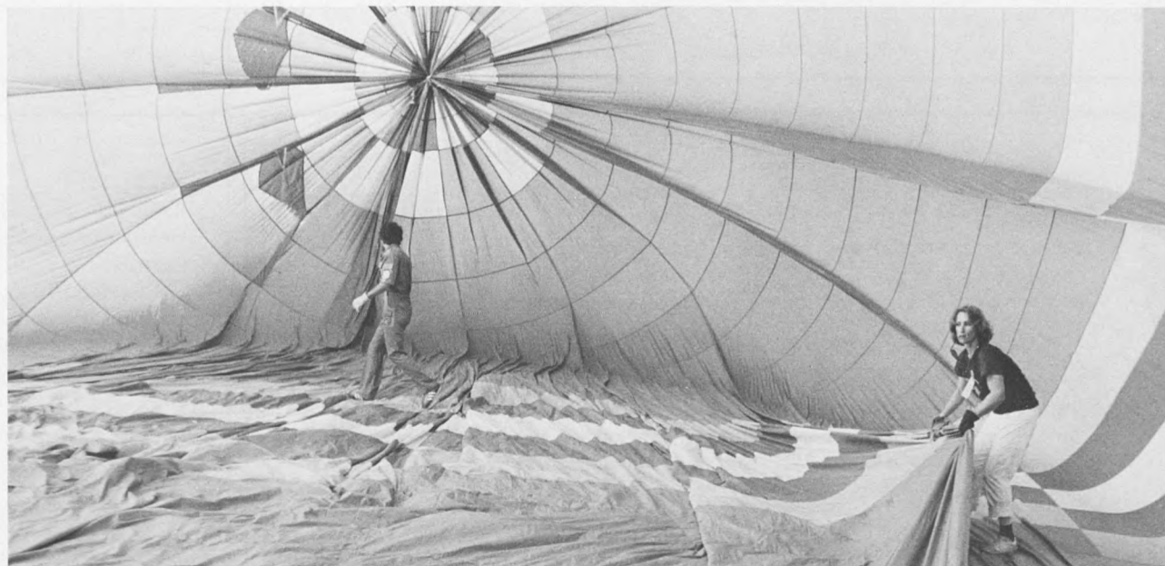
The balloon envelope is usually made of lightweight, tear-resistant rip-stop nylon which is reinforced with "rip stoppers" to check tears. An average envelope is made from over 1200 yards of fabric and could weigh as much as 120 pounds.
