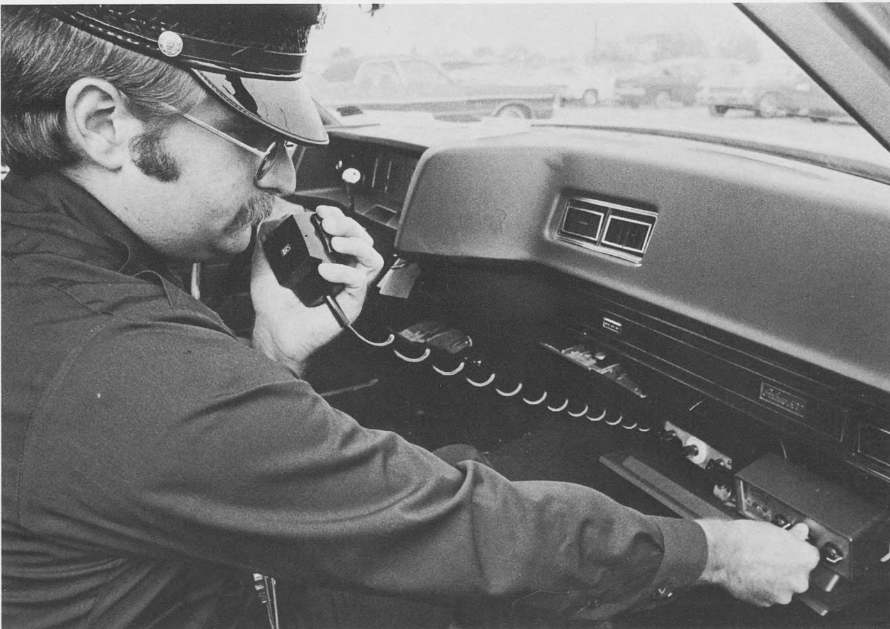
Jim McQue, security officer, checks the tuning of his CB radio with a meter designed to show most efficient operation.
