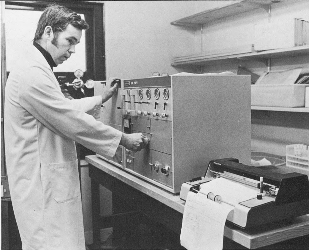
Dr. Marr demonstrates gas chromatograph. Printout of graph at right enables doctors to identify bacteria.
