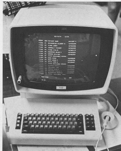
Cathode ray tube terminals aid in quickly identifying and locating available beds, thus speeding up the admitting procedure for both patients and hospital personnel.
