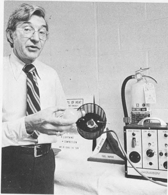
From left—Safety and Security director Ed Thurman inserts an ordinary light bulb into an electrical socket (protected by a metal cage) and sets it over a small metal skillet containing a few drops of gasoline. The light bulb is turned on, but
