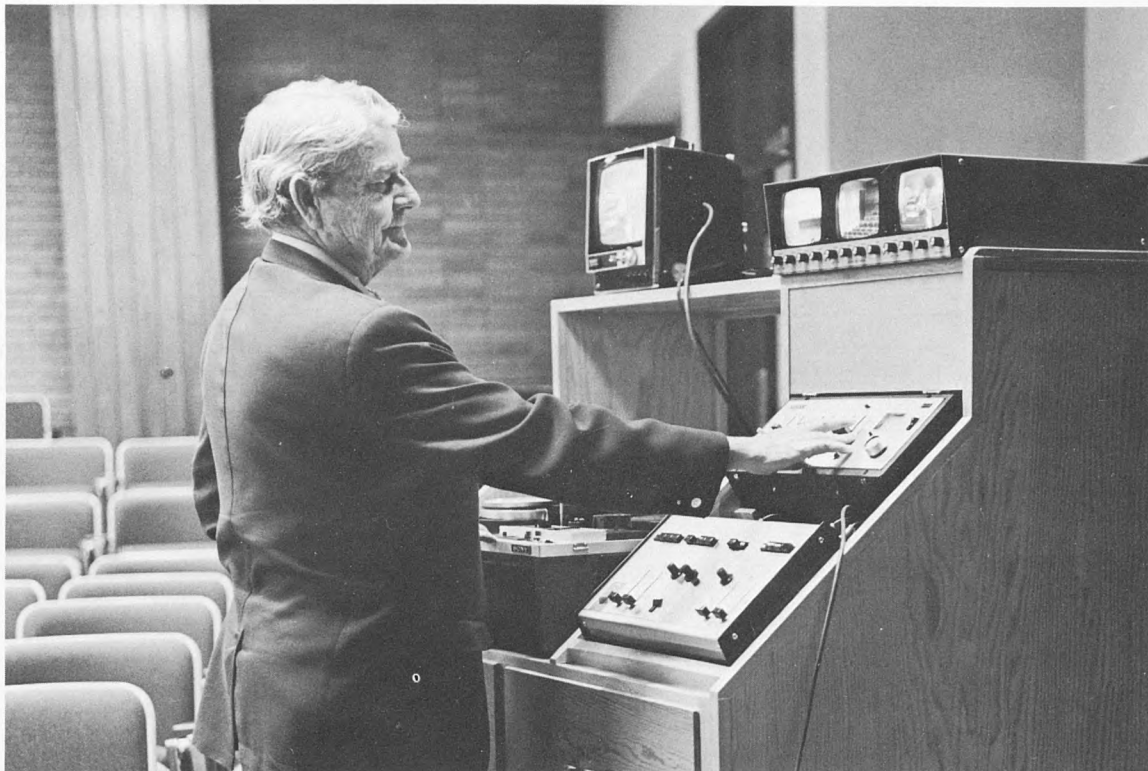
A videotape recorder, small TV monitors, and electronic switching and mixing controls are all mounted on a cart that can be moved from location to location. Storage space for TV cameras is also provided.
