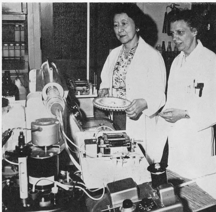
PREPARING THE AUTO ANALYSER for an experiment are Dr. Sue Stevens, left, and Miss Wilma White. Dr. Stevens holds the cylinder of cups, into which the urine samples are placed. The analyser removes the sample and runs it through a series of tubes where it is mixed with reagents. Then the intensity of the color of the sample is measured in a colorimeter, and this is automatically recorded.
