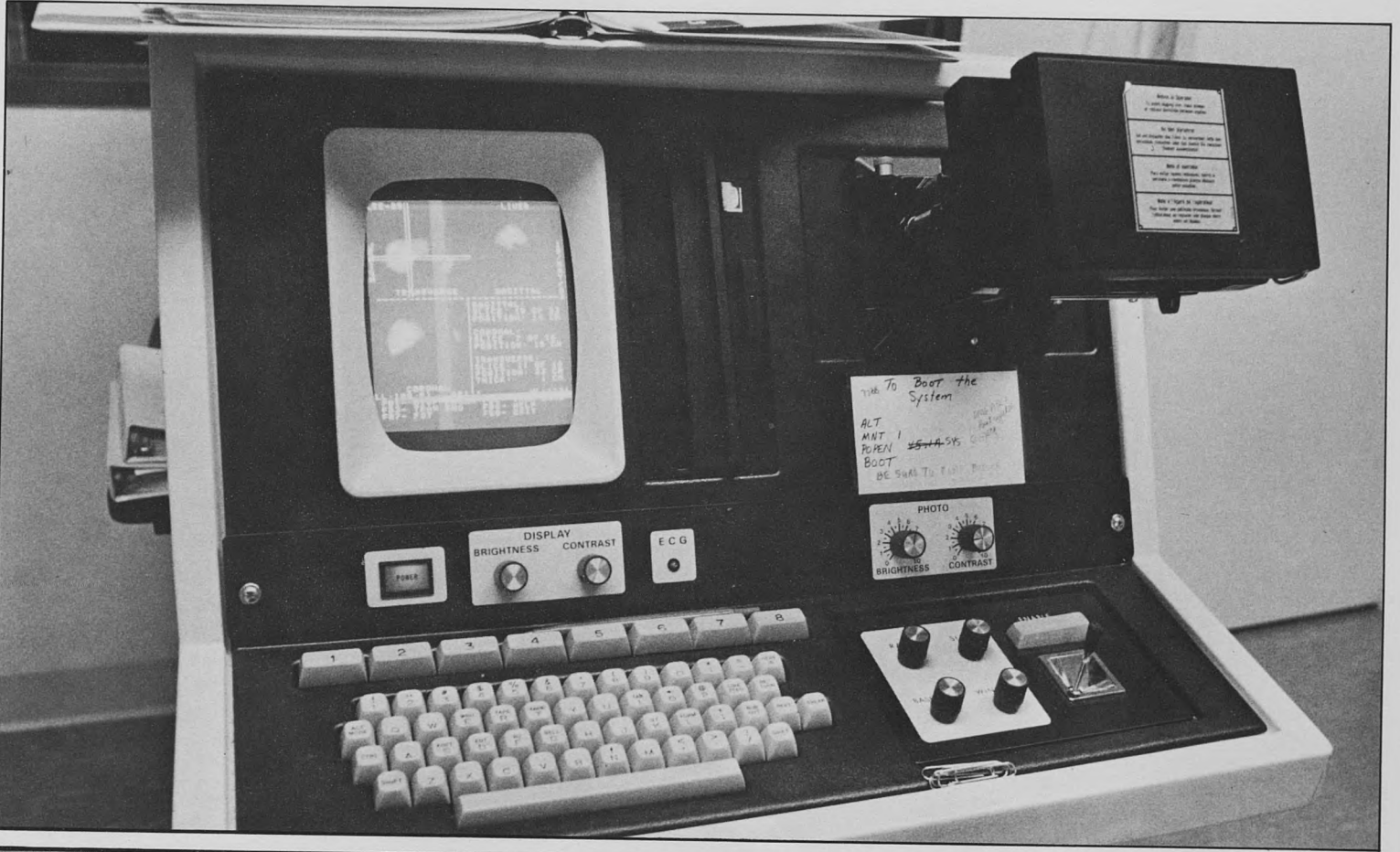
Three components make up the ECT machine. Other page: The control panel is housed in the room with the camera, at left. The computer, located in another room, is shown above with a cross-section on its screen.
