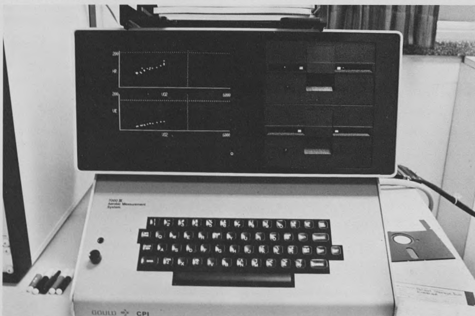
The computer module, able to produce graphic representations of patient performance data. The top graph shows oxygen used per heartbeat; the bottom graph reveals the ventilatory equivalent. Both are general fitness indicators.
