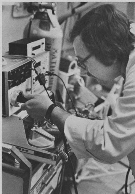
David Sinks, exercise physiologist in the Pulmonary Function lab, plugs in an oximeter prior to the exercise test. It will be used to compute the oxygen saturation in the blood during the test.
