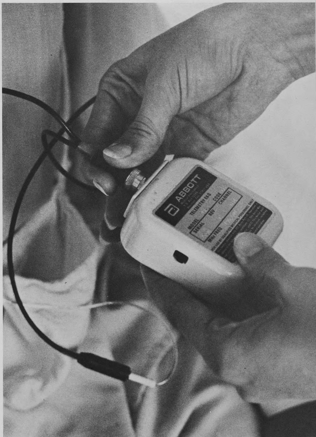
A lightweight battery-operated transmitter that is worn by the patient sends his electrocardiogram to the telemetry monitor.
