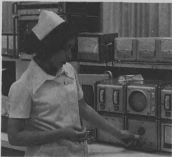
Miss Anna Babineaux, LPN, watches a heart monitor at the central station. Nine beds have cardiac monitors which continuously register heart rate and EKG pattern and signal when any unusual change occurs.
