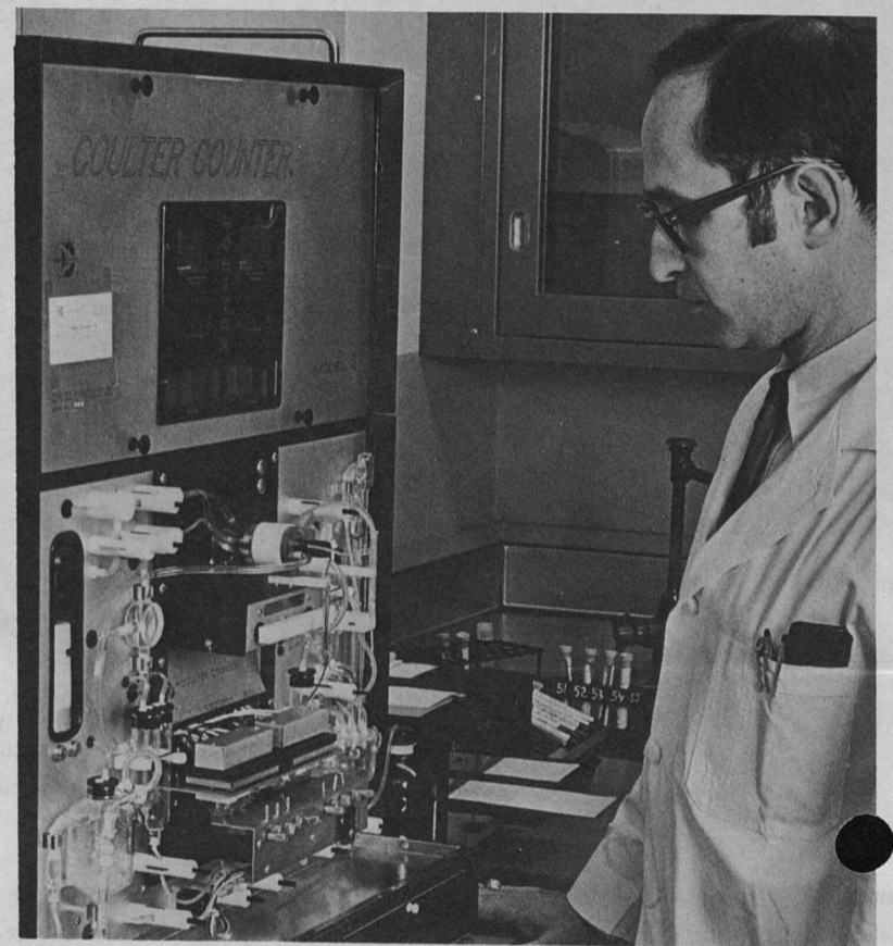
Herbert Silver, M.D., director, Hematology and Blood Bank in the Department of Pathology and Laboratory Medicine, examines the new push button Coulter Counter Model S, which provides seven different blood determinations in 40 seconds.
