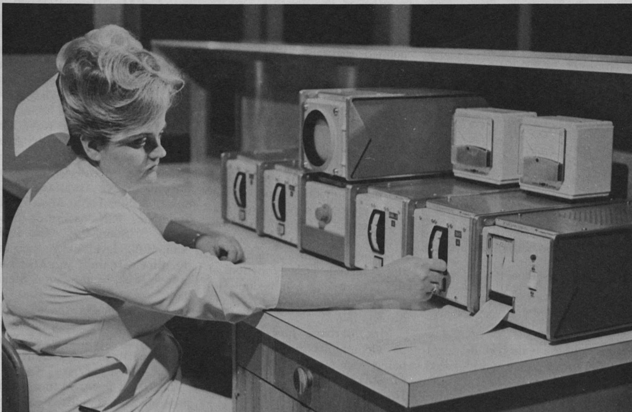
MISS ELSIE NULL, R.N., head nurse, Surgical Intensive Care Unit, adjusts heartbeat monitor limits on the "Parametron" unit. If a patient's heartbeat goes above or falls below certain limits, an alarm is sounded. Meters in the cases above the heartbeat monitor indicate blood pressure. The EKG recorder (instrument on the far right) records a patient's heartbeat if the alarm goes off or if the nurse activates it for some other reason.
