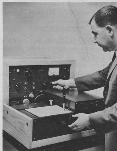
Testing dials on the new $3,000 Bekesy audiometer is Dr. Robert Goldstein, director of the Audiology section. The instrument, gift of the hospital Auxiliary, assists in determining hearing deficiencies of patients of all ages.
