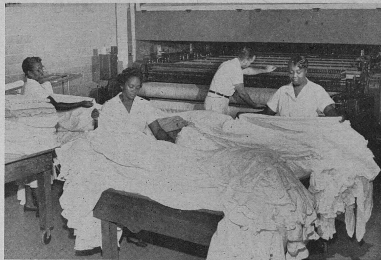
Preparing sheets for processing through the mangle shown in the background, which dries and irons linens preparatory to folding, are (left to right) Miss Julia C. Bradford, Miss Jessie L. Sykes, and Mrs. Elnora Levells. Mr. Freeman Burrow, Laundry Manager, checks operation of the mangle.
