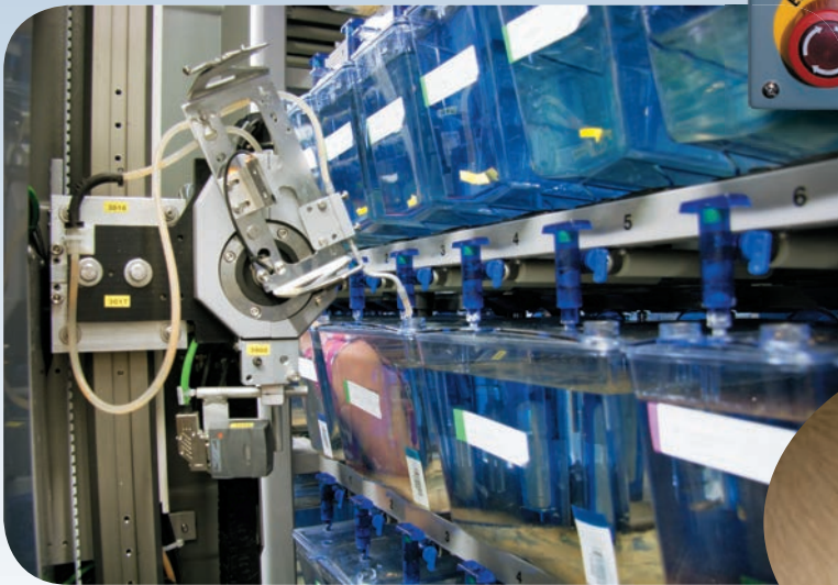
Large numbers of fish grow quickly as robotic feeding machines travel to each tank, providing frequent small meals.
