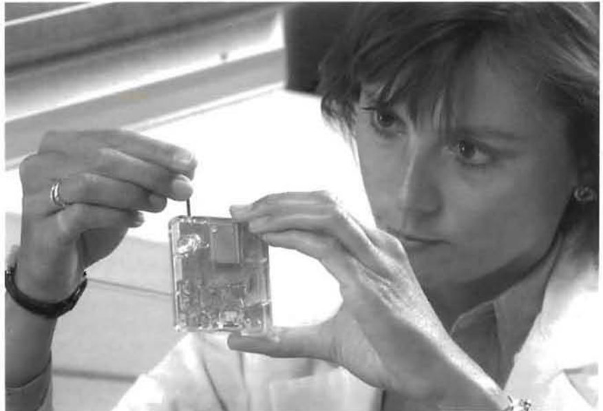
Sample holders in the Vision System, which separates whole blood into cells and plasma and then mixes a correct amount of plasma with reagents.
