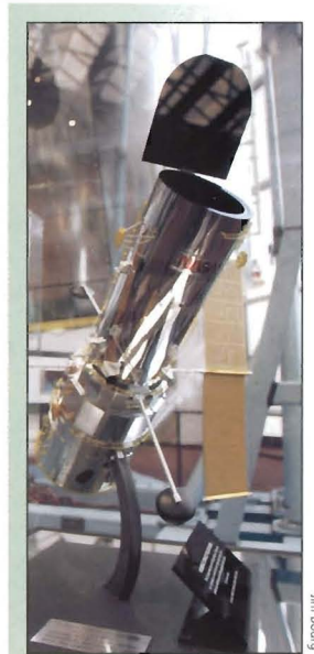
Polites did pioneering work in the use of magnetic torquers for spacecraft emergency stabilization and backup attitude control on the Hubble Space Telescope. This eliminated the need for a thruster system.
