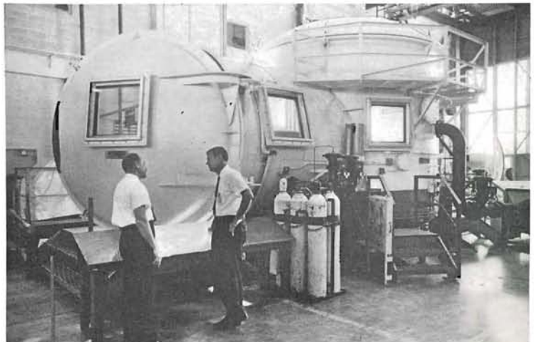
Altitude chamber in background is one of the many ingenious pieces of apparatus used to simulate conditions found in space. Within the chamber, it is possible to take "flights" hundreds of thousands of feet high.
