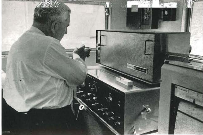
A sample of air is injected into a gas chromatograph, which will give an exact quantitative analysis of all volatile gases present.
