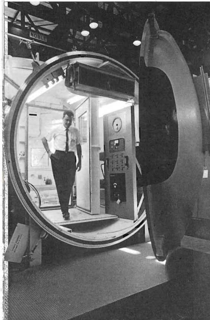
Yardley leaves the altitude-simulation chamber at Cape Kennedy. The chamber is used to test the astronauts and their equipment in conditions resembling those found at extreme altitudes above the earth.
