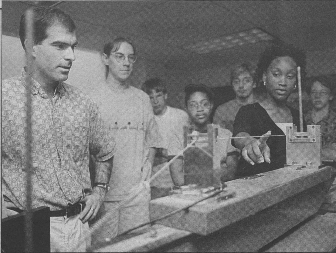
Excitation Philip V. Bayly, Ph.D. (left), associate professor of mechanical engineering, demonstrates for students from St. Louis' Metro High School the response of a string to excitation. The students examined oscillations by looking at the system with a strobe light, and thus observed a classic instance of nonlinear behavior. Students were on the engineering campus and at Boeing Co. laboratories for seven weeks this summer as part of the Boeing/Washington University Advanced Manufacturing Research and Development program with the school, intended to expose bright students to engineering careers. Jerry Halley, a Boeing employee and Bayly's graduate student in mechanical engineering, coordinated the program.
