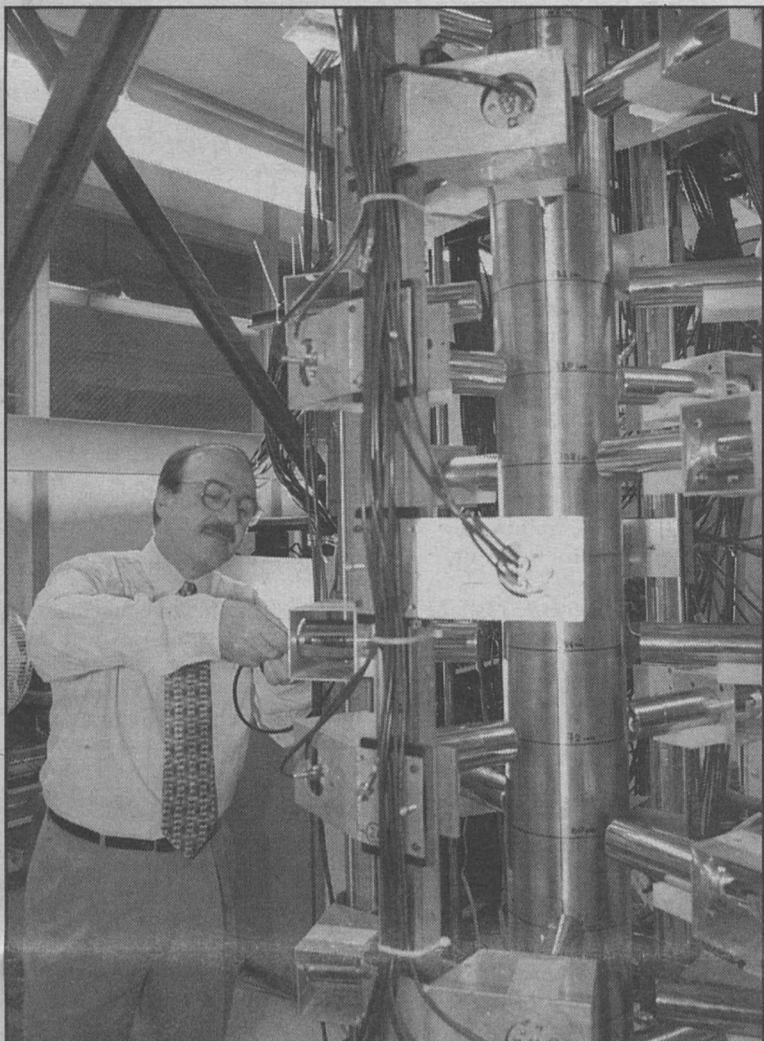
Muthanna H. Al-Dahhan, Ph.D., assistant professor of chemical engineering and associate director of the Chemical Reaction Engineering Laboratory, inspects a slurry bubble column reactor, the reactor of choice for a wide range of industrial processes, including ways to produce alternative fuels from coal.
