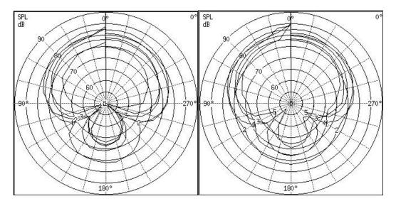
Figure 4: An example of a hearing aid that shows minimal change in both the FSR calculation and graphic representation of polar plots between the initial measurement (a) and the follow up measurement 3 months later (b).
