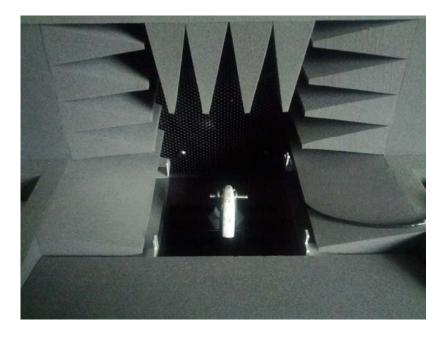
Figure 2a: Traditional BTE hearing aid connected to an HA-2 coupler
