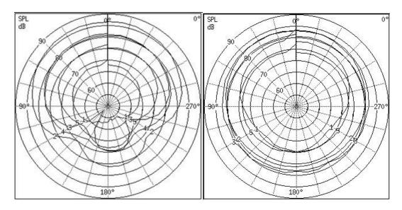
Figure 5: An example of a hearing aid that shows remarkable change in both the FSR calculation and graphic representation of polar plots between the initial measurement (a) and the follow up measurement 3 months later (b).
