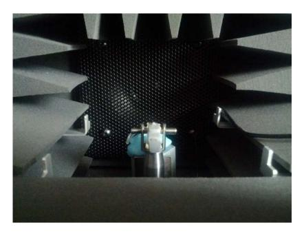
Figure 2b: RIC BTE hearing aid connected to an HA-1 coupler
