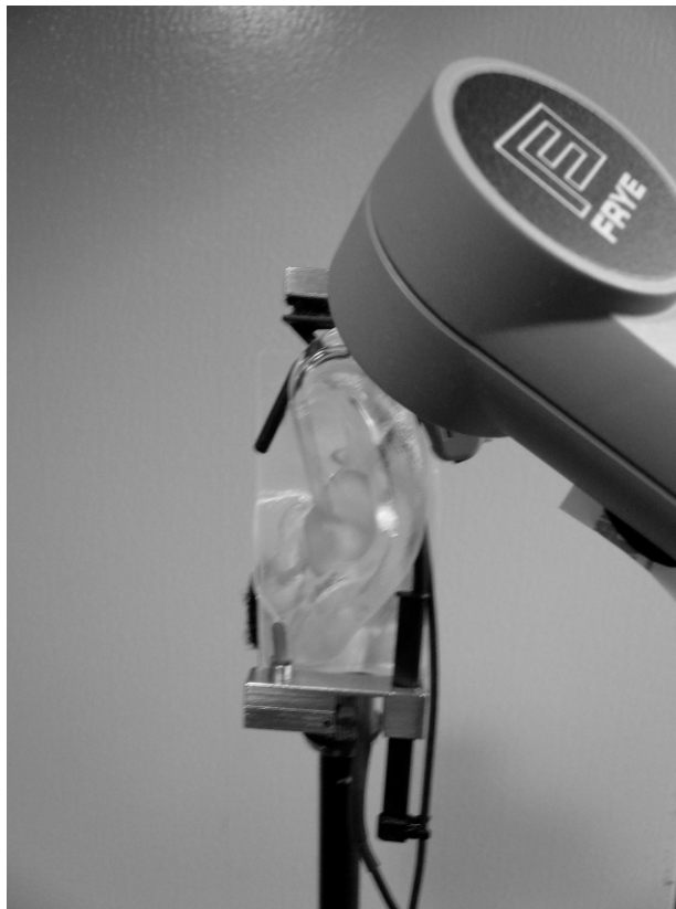
Figure 7: An FP40 telewand (Frye Electronics, Inc.) positioned to transmit the DigiSpeech signal to the t-coil of the test BTE for real-ear t-coil frequency response measure.
