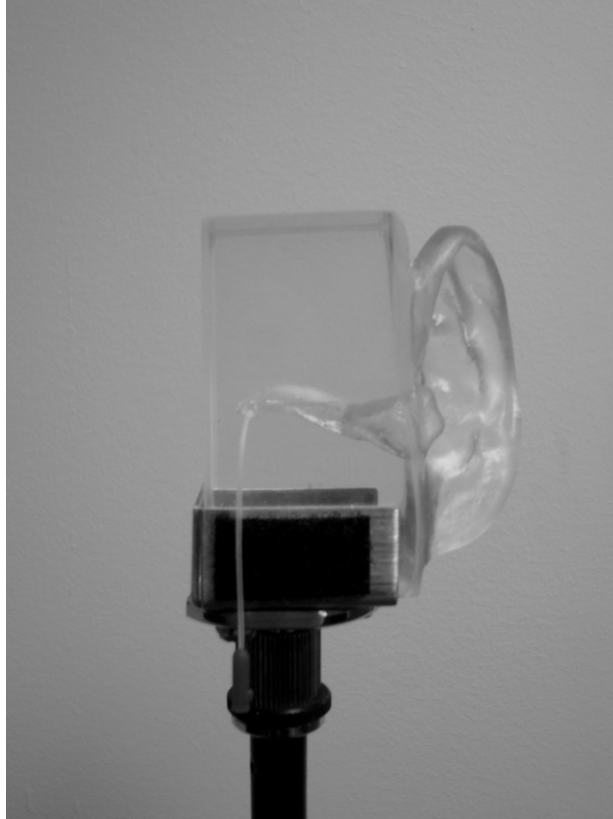
Figure 4: A coronal view of the dummy ear (Frye Electronics, Inc.) mounted on a tripod with a probe tube fed through a bored hole and into the medial external auditory meatus (EAM).
