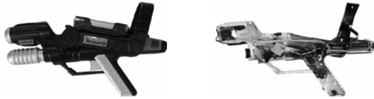
Figure 3: (a) A complete handset with iPAQ; (b) Cut-away view of the handset showing GPS, compass, trigger and battery.
